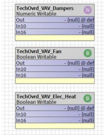
2. Locate the folder where the components to be overridden are located in the NavTree and select the Wiresheet View, then right click on the folder on the Wiresheet and select COMPOSITE to exposed the composite editor and add the relevant inputs
